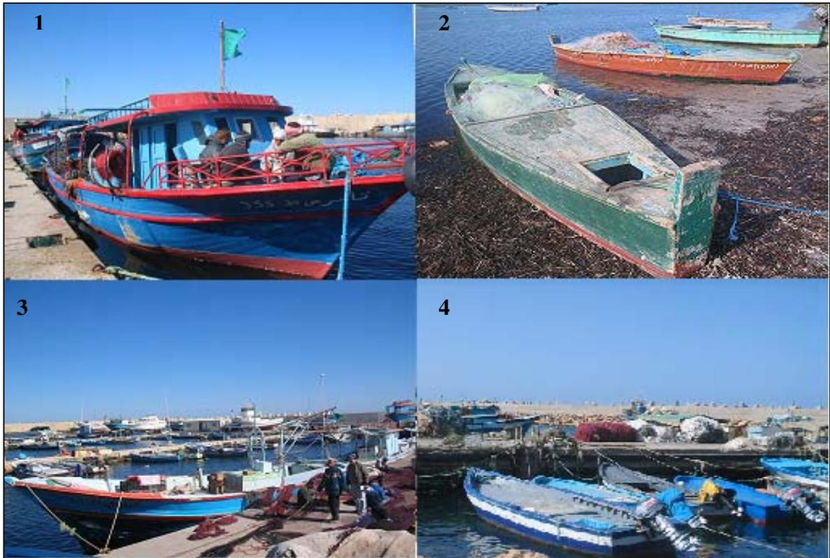
**Fig. 2.** The fishing vessels used along the Libyan coast: 1 Mator, 2 Batah, 3 Lampara, 4 Flouka.
